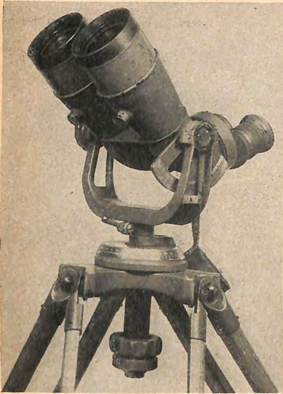
Figure 312. Model 89 (1929) 10-cm AA spotting binoculars.
